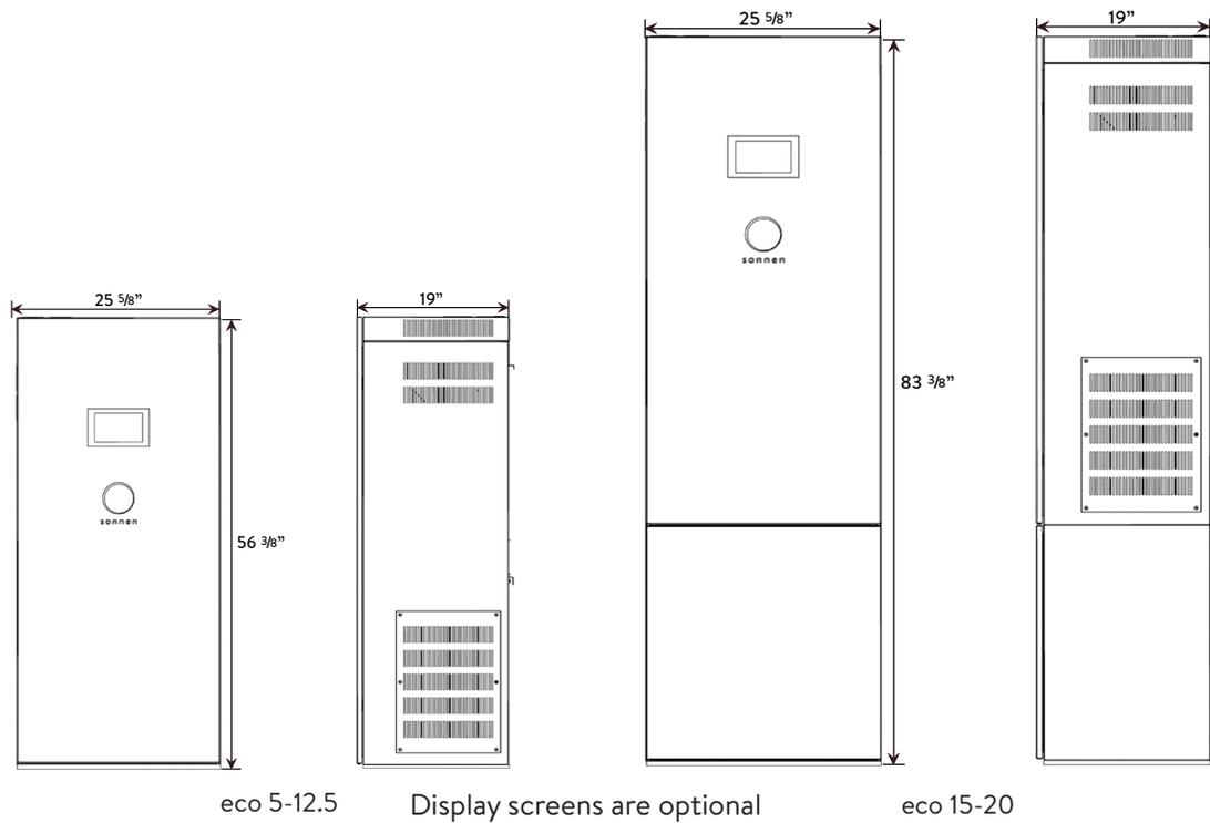
Fig. 2 Storage system dimensions
