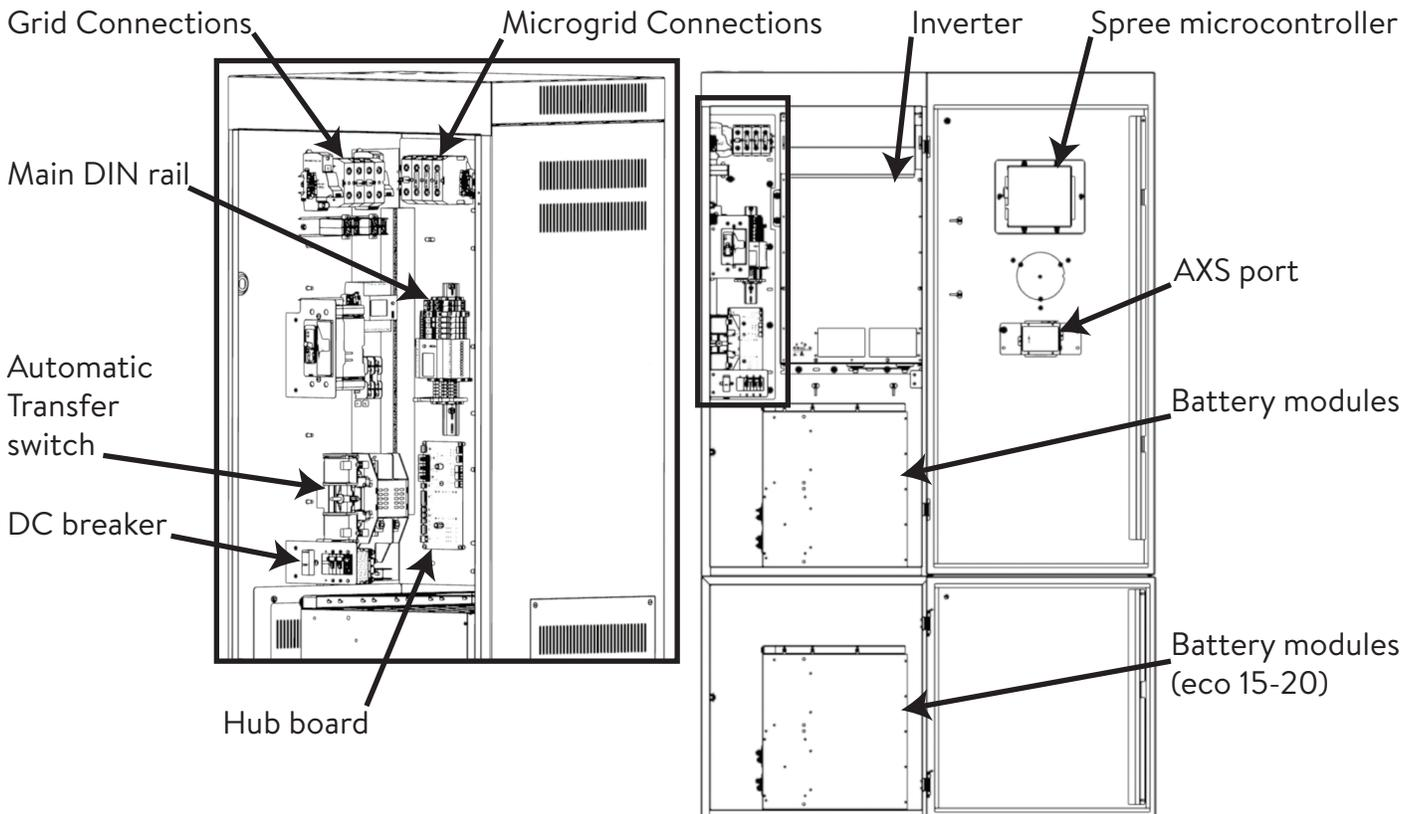
Fig. 3 eco Gen 3.1 key components
