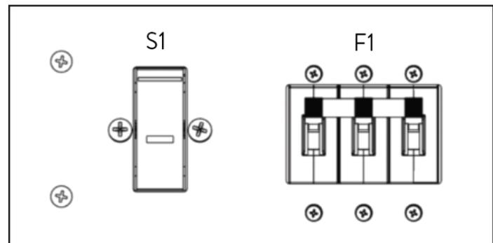
Fig. 9 Pre-charge switch and circuit breaker
