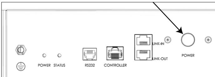
Fig. 8 Battery module power button
